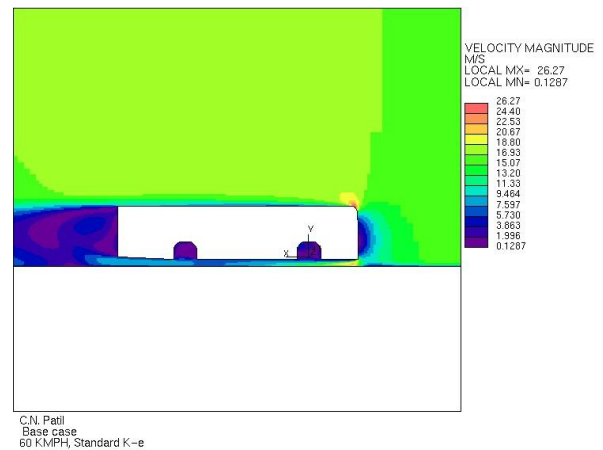
Figure 7: Velocity plots at mid section of Base Model
