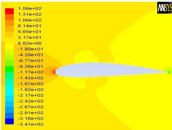
Fig.20 Pressure Plot – 10^\circ Angle of attack
