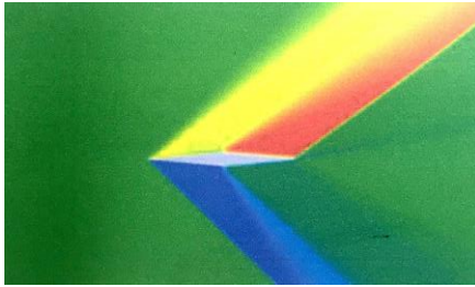
Figure 12 Expansion wave observed at top leading edge
