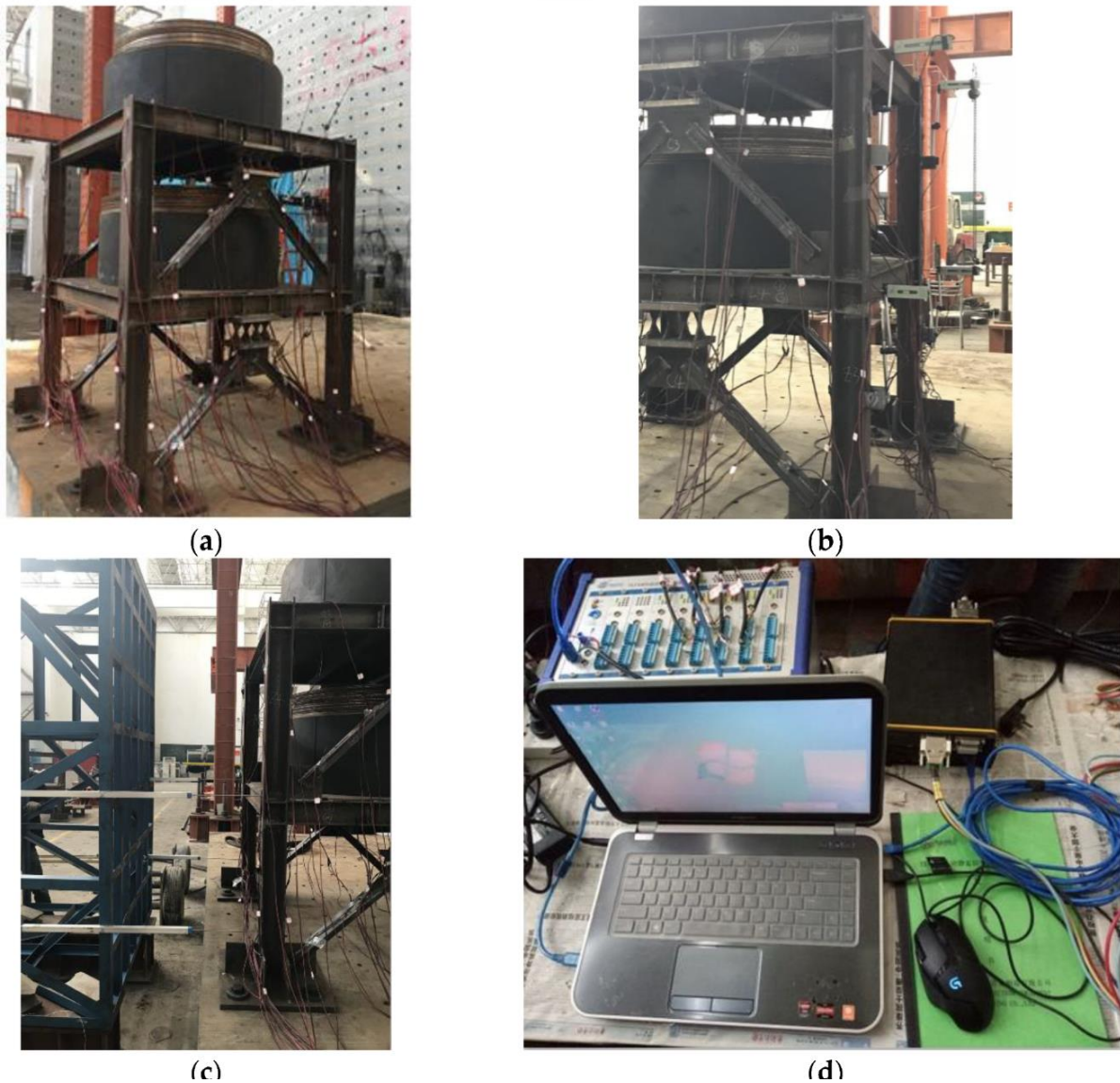
Fig. 9. Measuring devices of the specimen. (a) Connection of strain gauges; (b) YHD sensors; (c) TST sensors; (d) data acquisition instrument [39].
