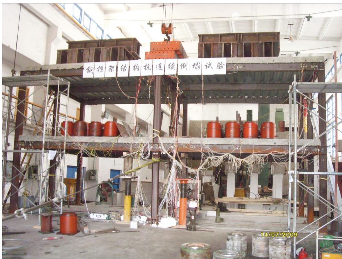
Fig. 6. Test setup of the two-story steel frame [ 27].
