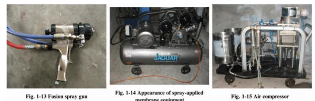
Fig. 7. Spray-applied membrane equipment and system
