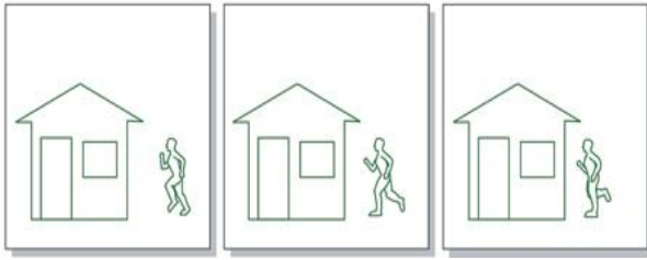
Figure 3: With the Motion JPEG format, the three images in the above sequence are coded and sent as separate unique images (I-frames) with no dependencies on each other.
