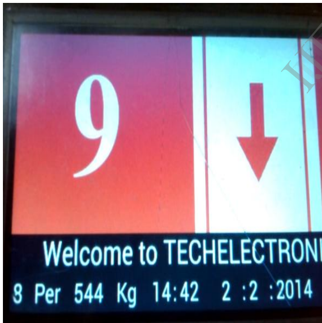
Figure3: TFT display showing final output of the system.
