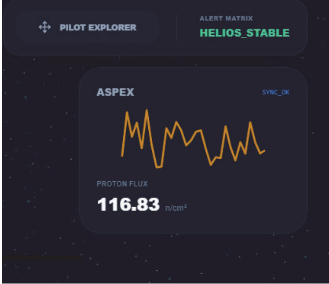
Fig. 8: ASPEX Solar Wind Particle Spectrometer Telemetry Card (Proton Flux = 116.83 n/cm 2 ). The amber-gold waveform encodes the instantaneous solar wind proton number flux. The elevated reading ( \approx 2\times quiet-sun peak) is consistent with an interplanetary shock arrival. The Frozen-in Flux theorem [27] dictates that elevated proton flux arriving simultaneously with southward B_z constitutes the primary cross-instrument trigger for the CatBoost ICME shock classifier. Rolling dN/dt and d^2N/dt^2 features distinguish genuine shock ramps from corotating interaction region (CIR) density fluctuations.
