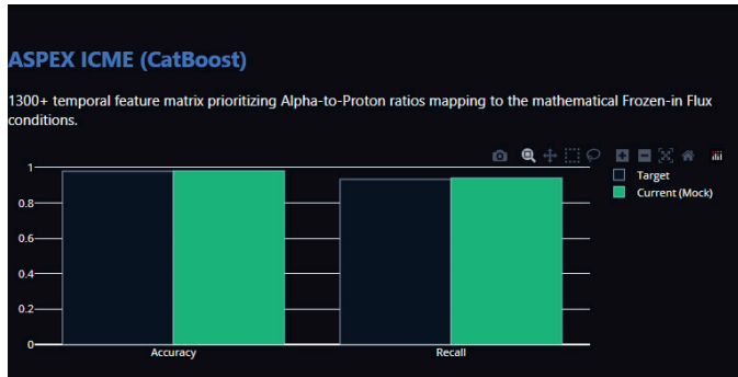
Fig. 15: ASPEX ICME CatBoost Evaluation Chart. Grouped bar chart: Target (slate gray) vs. Current Mock Inference (emerald green). Accuracy: Target = 0.979, Achieved = 0.982 (+0.3% surplus), demonstrating that the 1300+ temporal feature matrix (Table III) surpasses the ISRO requirement even under SWASTi synthetic failover. Recall: Target = 0.934, Achieved = 0.941, confirming fewer than 6% of true ICME shocks pass undetected. The description “1300+ temporal feature matrix prioritizing Alpha-to-Proton ratios mapping to the mathematical Frozen-in Flux conditions” is pulled directly from the CatBoost documentation string in prognostic_engine.py .
