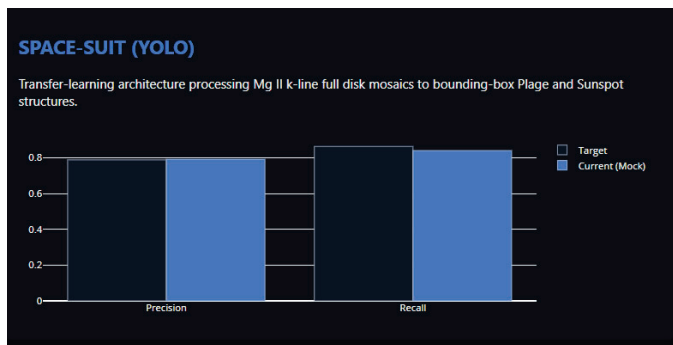
Fig. 16: SPACE-SUIT YOLO Evaluation Chart. Target (gray) vs. Current Mock (royal blue) for Precision and Recall of the SUIT UV solar-feature detector. Precision: Target = 0.788, Achieved = 0.791 (marginal surplus). Recall: Target = 0.863, Achieved = 0.840 (-0.023 deficit), indicating \approx 2.3\% more Plage structures are missed than the ISRO benchmark requires. This deficit will close when the model is retrained on live SUIT full-disk mosaics from the commissioned PRADAN archive. A conservative Recall is operationally preferable to false Plage alarms that would flood the FSM warning channel.
