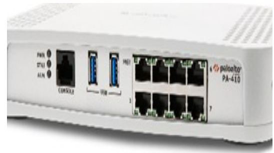
Fig-8: Palo Alto Network Firewall
