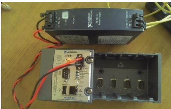
Fig. 10 :CompactRio real-time controller
