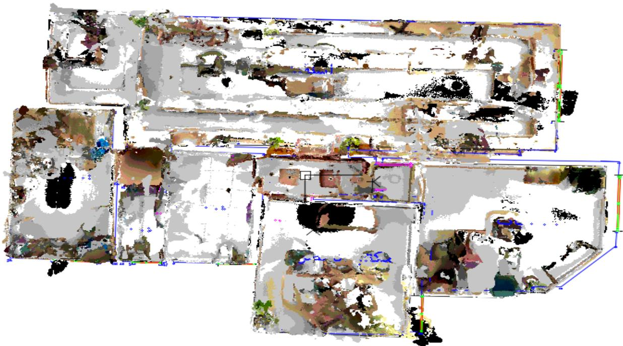
Figure 1: 3D point cloud as produced from iPhone scanning
