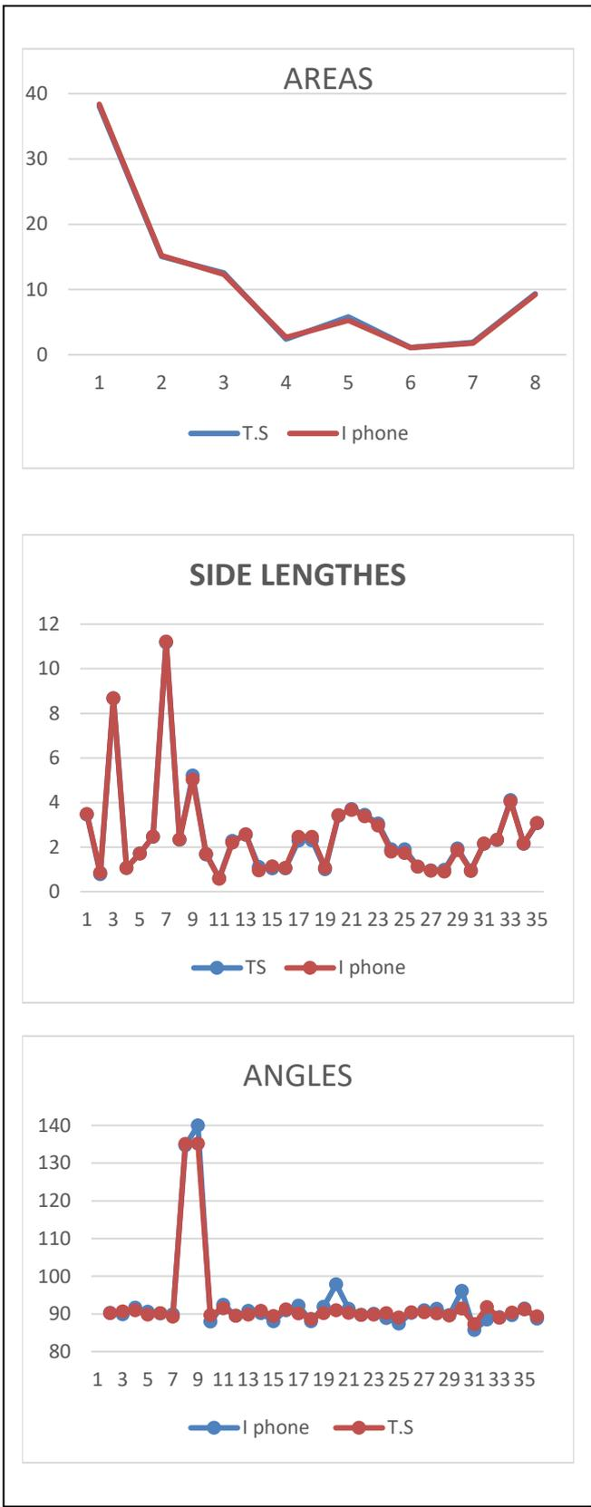
Fig. 12: A profiles for Areas, Side lengths and Angles for the 2D plan produced from TS and iPhone LiDAR.
