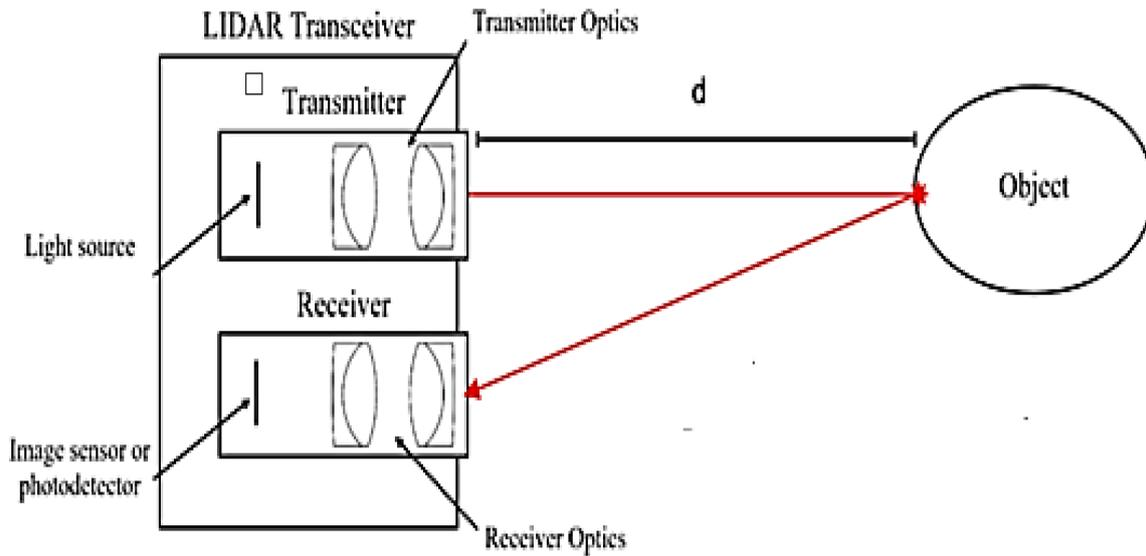
Figure 1: principal of laser scanner
