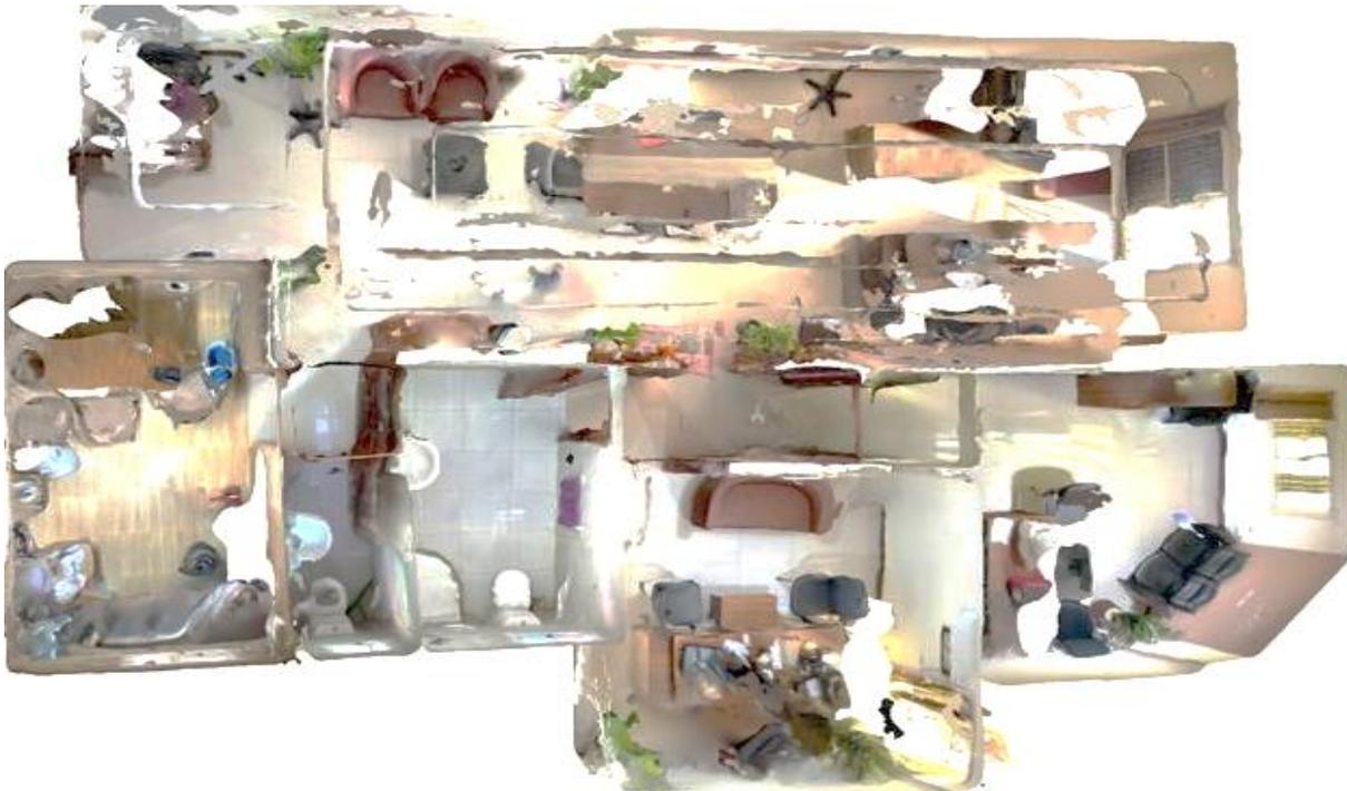
Figure 2: 3D modeling produced from point cloud after process.
