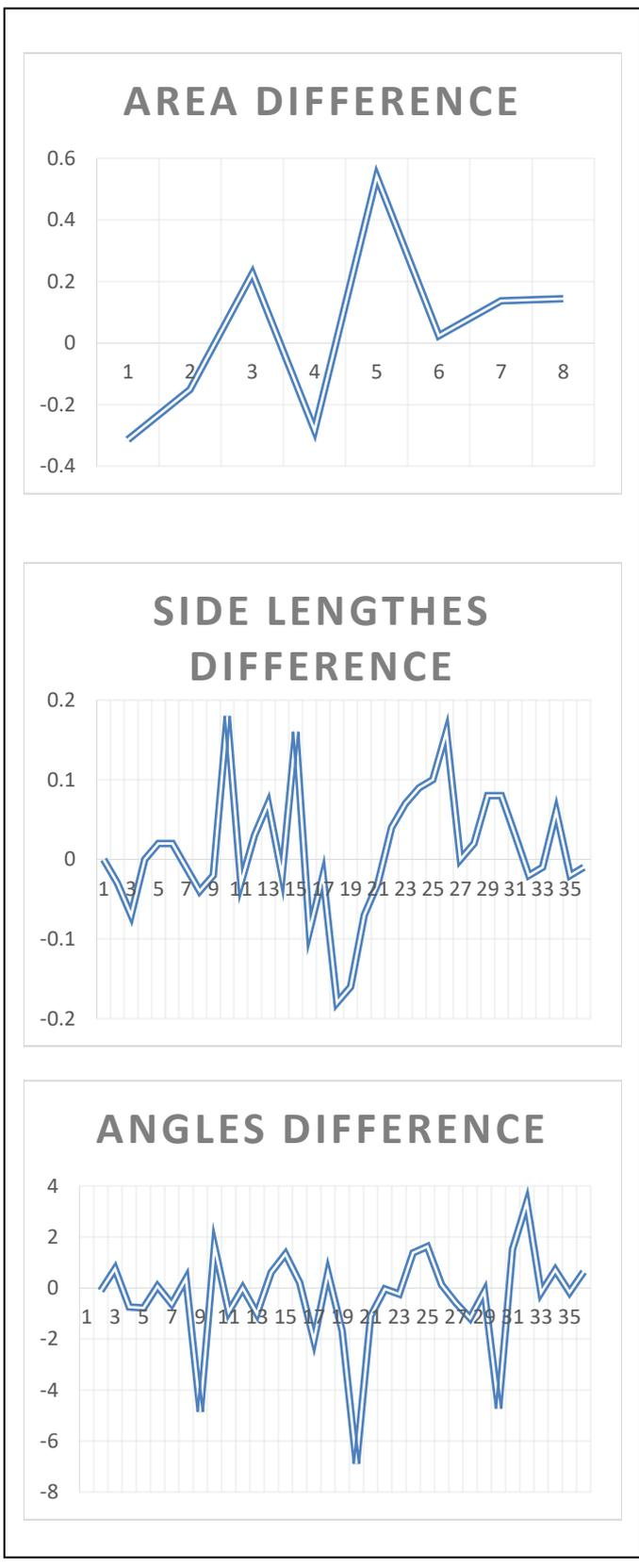
Fig. 13: A profiles of differences for Areas, Side lengths and Angles for the 2D plan produced from TS and iPhone LiDAR.
