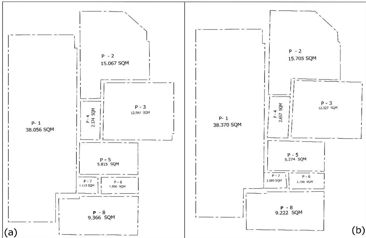
Figure 9: 2D plan indicates partitions areas, (a) produced from I phone and (b) produced from total station.
