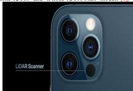
Figure 2: LiDAR scanner location in I phone mobile.
