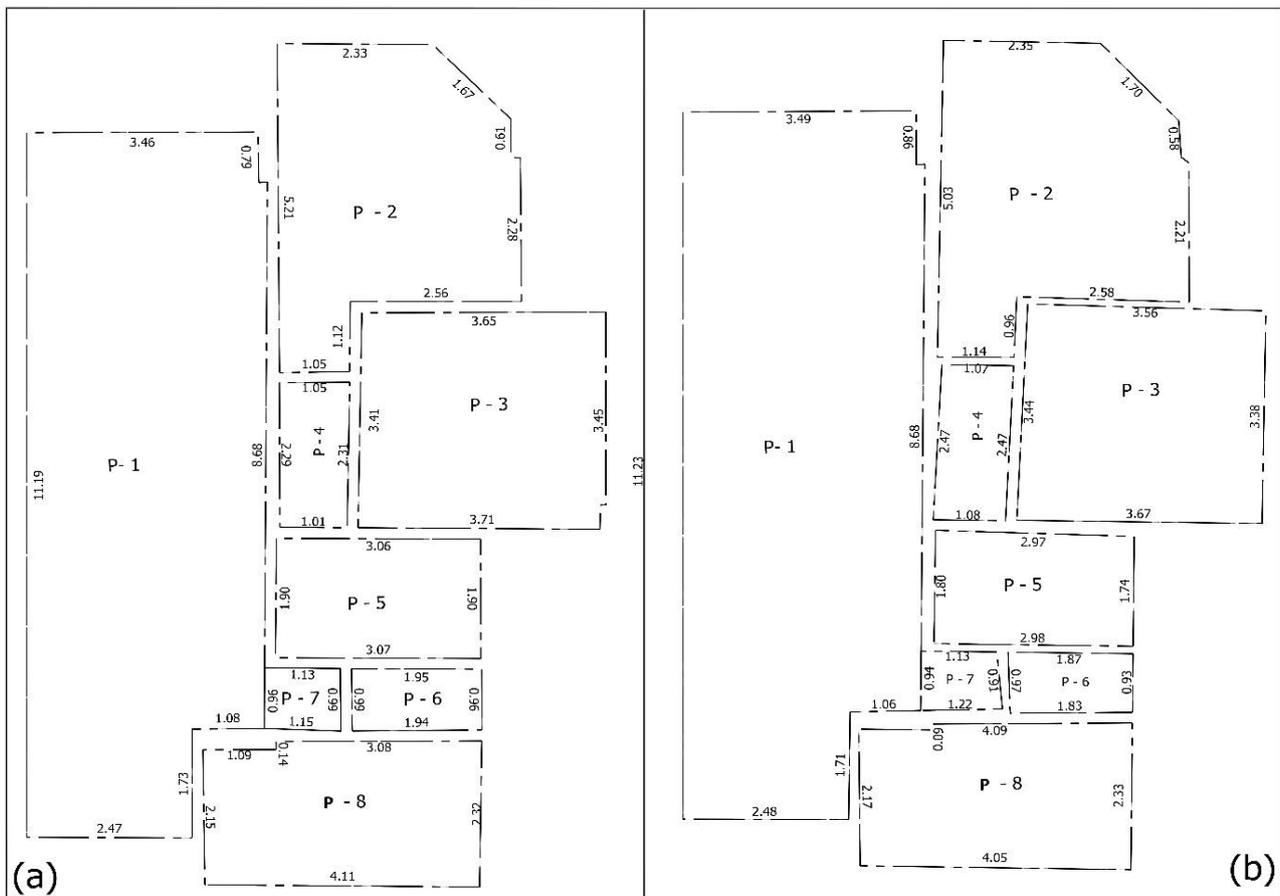
Figure 10: 2D plan indicates side lengths, (a) produced from I phone and (b) produced from total station.
