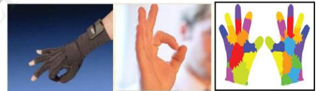
Fig. 1 (a) Data Glove based, (b) Vision based, (c) Colored marker based (From web gallery)
