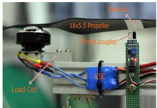
Figure 1 Sensor Configuration [3]
