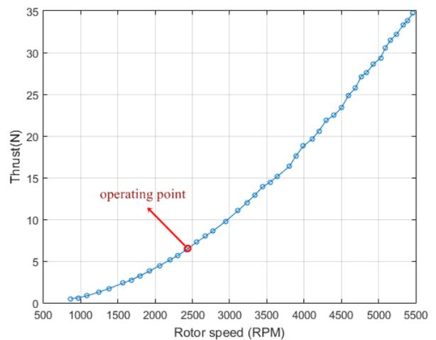
Figure 4 Thrust versus Speed
