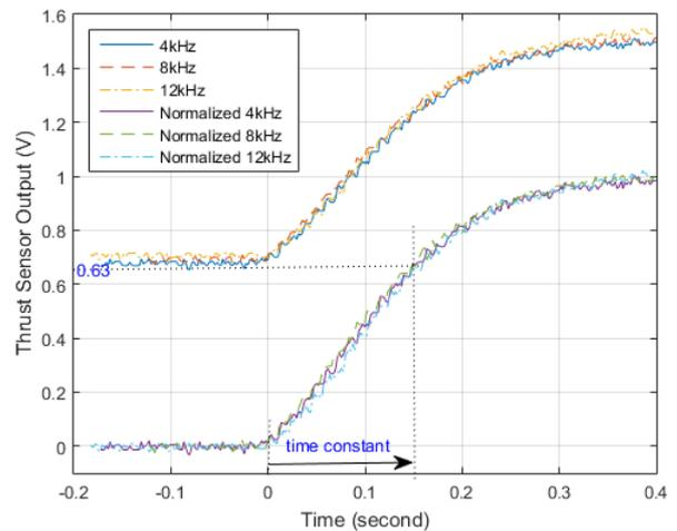
Figure 5 Thrust Step Response [1]
