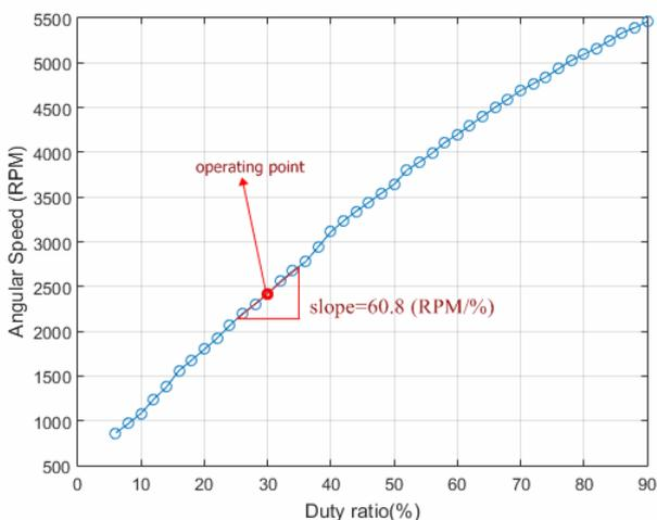
Figure 2 Speed versus Duty Ratio
