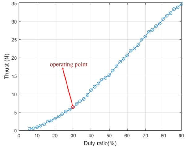
Figure 3 Thrust versus Duty Ratio
