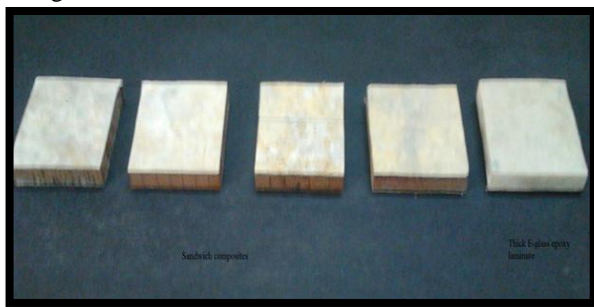
Figure 5.4 thick sandwich composite plates and E-glass epoxy laminate
