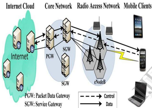
Fig.1.: Cloud Mobile Media architecture, showing control and data flows.
