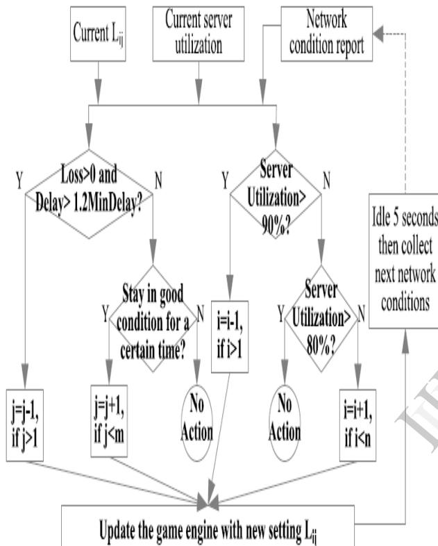
Fig 4: Work flow of level-selection algorithm
