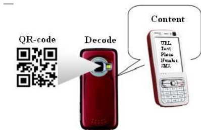
Figure 2 :QR-code Decoding diagram
