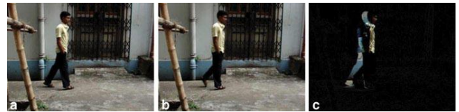
(a) Present frame (PF) (b) previous frame (prev) (c) result=PF-prev
