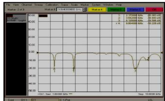
Fig. 5 Plot between return loss and frequency for Pentagonal Fractal Antenna
