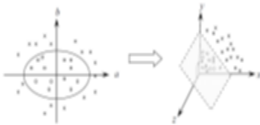
Figure 2: Kernel (nonlinear) mapping of 2-dimensional data into 3-dimensional space by polynomial kernel function. In the following, a brief introduction to several non-linear dimensionality reduction techniques will be given.
