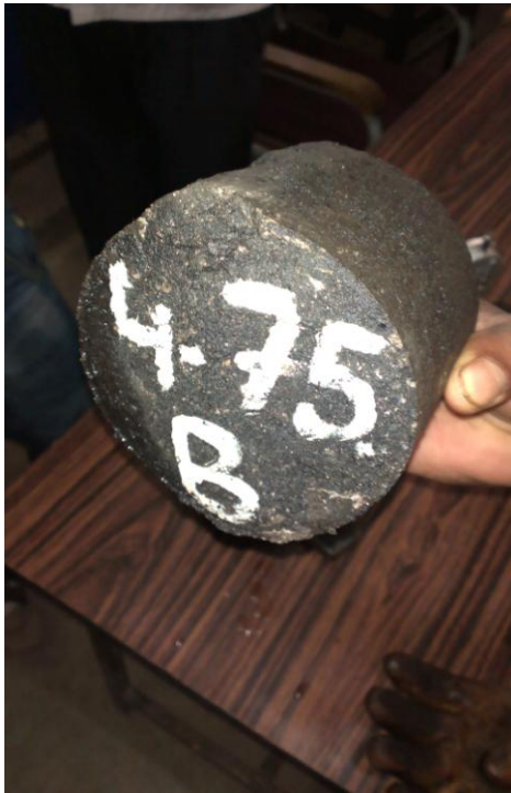
Figure 5: failed or bulged mould after testing.
