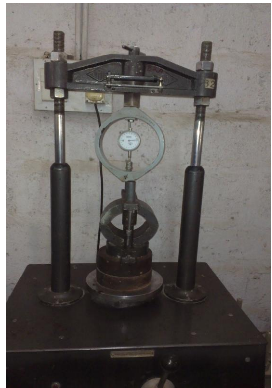
Figure 4: placing a mould inside the breaking head for testing.
