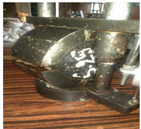
Figure 4: placing a mould inside the breaking head for testing.
