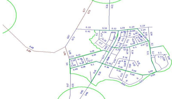
Fig. 19. Traffic possibility factor (v/c) under solutions 1 and 2 + Nguyen Van Tang route: belongs to LOS C and D - Traffic flow is relatively stable. + Nguyen Xien route: belongs to LOS C and D - Traffic flow is relatively stable. + Phuc Thien route: belongs to LOS A, B - Stable traffic flow, good driving condition.
