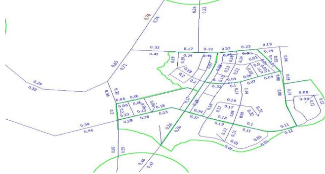
Fig. 20. Traffic possibility factor (v/c) when combining 3 solutions Level of service: + Nguyen Van Tang route: belongs to LOS C - Stable traffic flow. + Nguyen Xien route: belongs to LOS C and D - Traffic flow is relatively stable. + Phuc Thien route: belongs to LOS A, B - Stable traffic flow, good driving condition.
