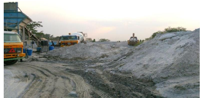
Fig. 1 Waste concrete dumped in RMC plant
