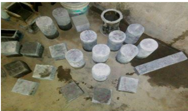
Fig. 3: Concrete cubes (150X150X150mm); Cylinders (150X300mm); Prism (500X100X100mm)
