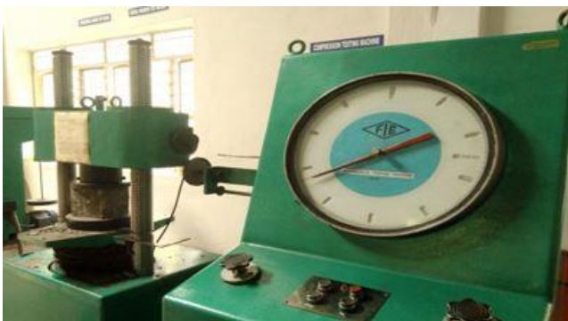
Fig. 2: Compressive strength test set up
