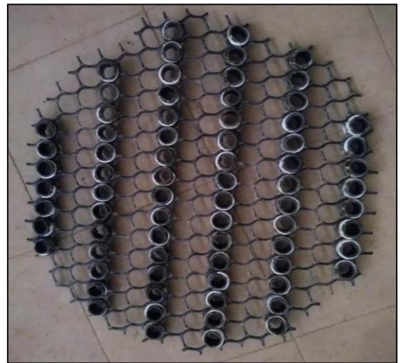
Fig 1: Layer of Geogrid-PVC Pipe
