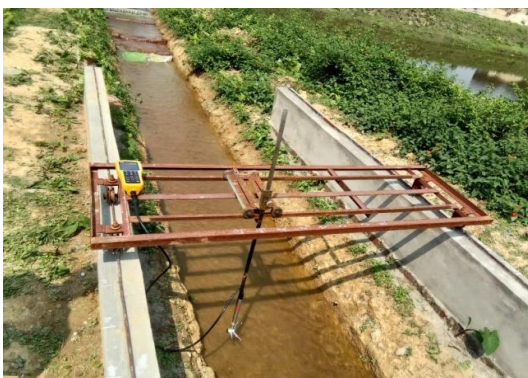
Fig 5: The ADV with probe over the steel trolley installed in the channel
