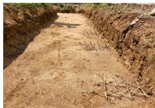
Fig 3: The prepared field channel with the installed porcupine models
