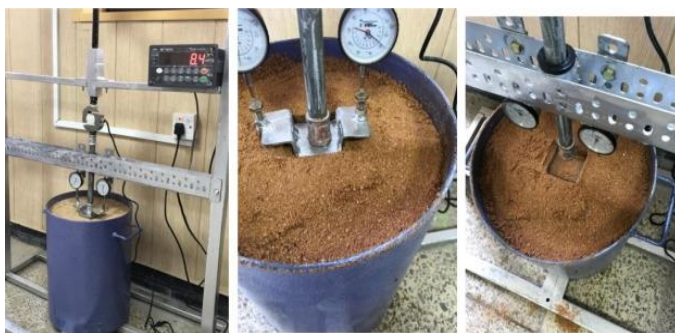
Fig.2 Load test on model footing
