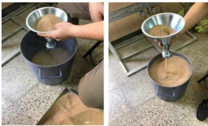
Fig.1 Sand bed preparation
