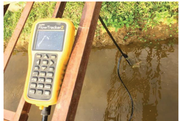
Fig 5: The ADV with probe over the steel trolley installed in the channel
