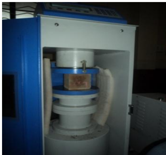
Fig 2. Compressive strength test
