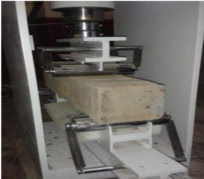
Fig 4. Flexural strength Test
