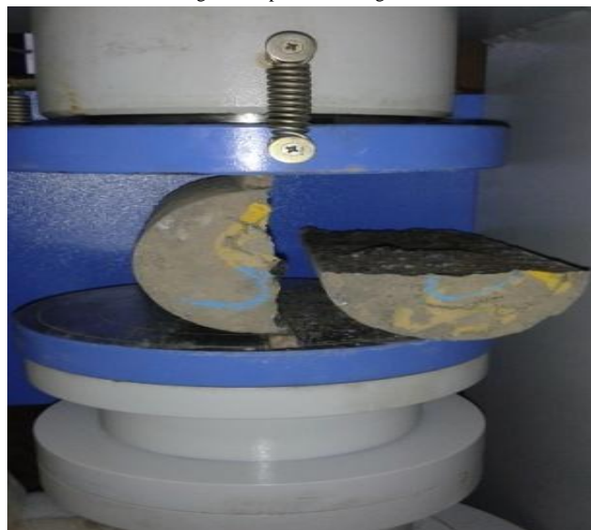
Fig 3. Split Tensile strength test
