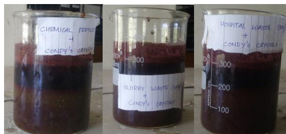
Figure 1. Soil Samples mixed with Condy's Crystals
