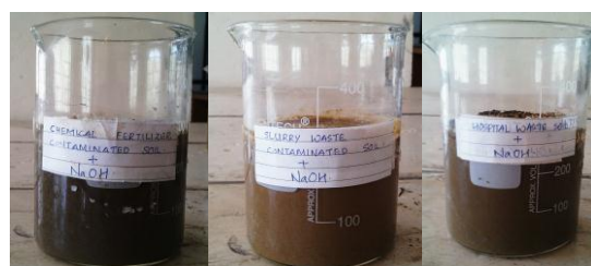
Figure 2. Soil samples mixed with NaOH
