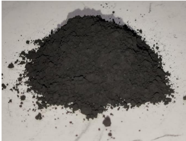
Commercial charcoal powder after standardized to the particle size of 75 microns
