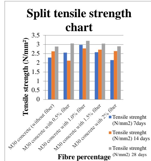
From the above bar chart it was observed that, the From the test results it has been observed that for M30 grade concrete the split tensile strength at the age of 7, 14 and 28 days are represented
