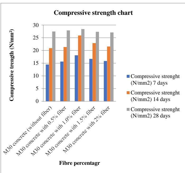
From the above bar chart it was observed that, the compressive strength test results of sisal fibre reinforced concrete, the sisal fibres are added to the concrete in varying percentage of 0%, 0.5%, 1%,
