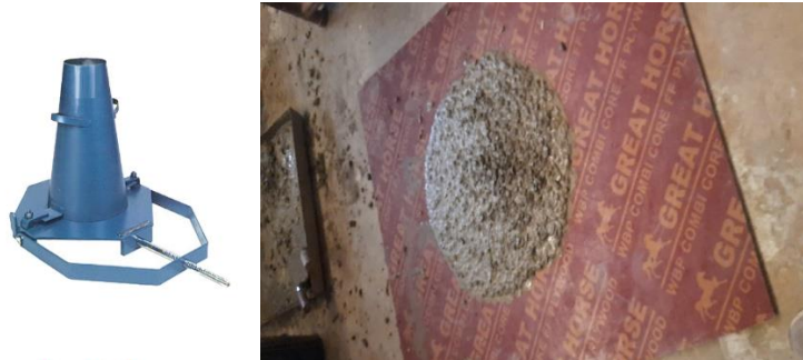
Figure 1: Slump Flow Test with Apparatus
