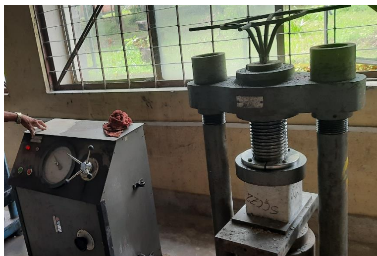
Figure 4: Compression Test on Hardened Concrete
