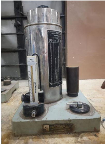
Fig. 5. Testing of Permeability using Permeability Meter
