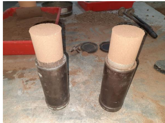
Fig. 3. ASTM standard Compressive and Permeability test specimens
