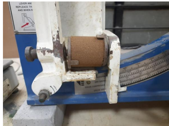
Fig. 4. Compressive strength testing using Universal Strength Machine
