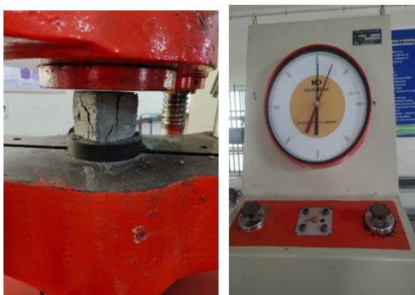
Fig 8: Compressive strength test of cube specimens
