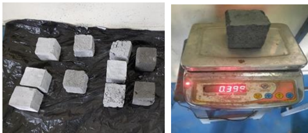
Fig 7: Cubes dried and density is determined
