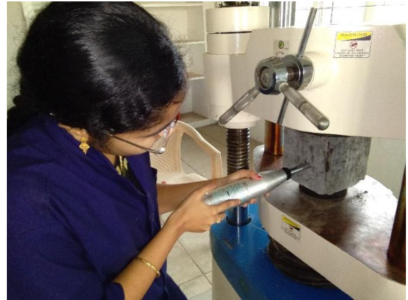
Fig2: Conducting Rebound hammer test
