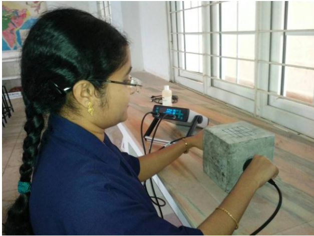
Fig1. Conducting ultrasonic pulse velocity test
