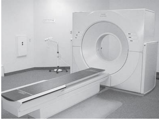
Fig 7(a) Outside view of third-generation CT scanner showing the patient table and gantry aperture.
