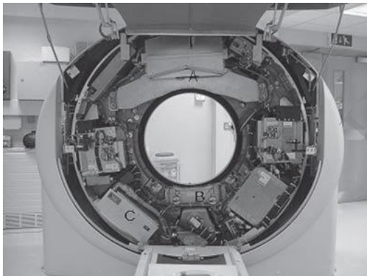
Fig 7(b) When the cover is removed, the x-ray tube and the arc of detectors can be seen. The gantry holding the x-ray tube and detector rotate around the patient as the data are gathered
