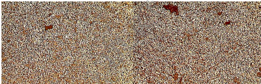
90% of aluminum, 2% of graphite, 6% of silicon carbide and 2% of boron carbide
