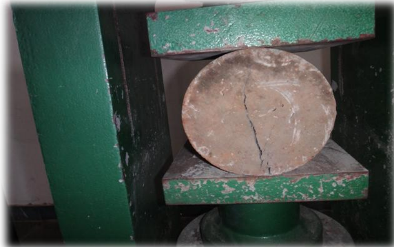
FIG II: Split tensile strength (f_s) = (2W)/(\pi LD)
