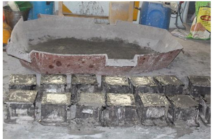
Figure 2: Casting of cubes
