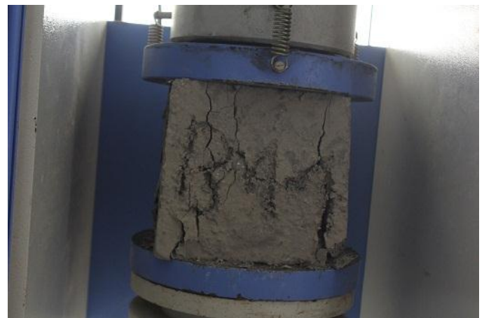
Figure 4 Failure pattern of cube
