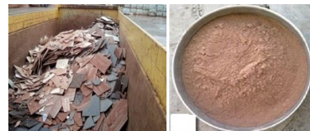
Fig.1. ceramic preparation process: (a) raw ceramic ground and grinded by hammer mill, (b) grinded by tabin crusher, and powdered by tabin mill.
