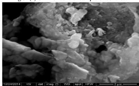
Fig 5 (b) SEM of sample containing 3% Nano-SiO 2
