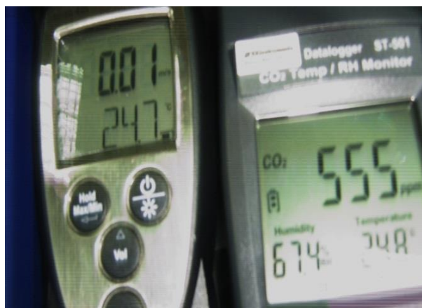
Fig. 4. Instrument used in this investigation Left (Anemometer-thermometer), Right (CO2 Temp/Rh Monitor)
