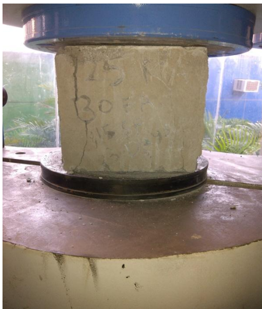
Figure 5.1 Compression Test on Cube (After Application of Load)
