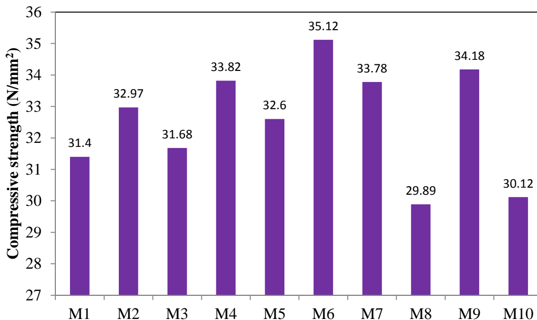
Figure 5.4 Compressive Strength of Concrete cubes after 28 days of Moisture Curing.
