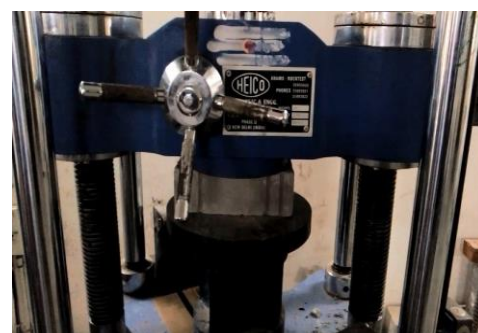
Fig 6. Compression testing of brick
