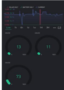
Fig. 9. Plot of solar voltage, battery voltage and current using Blynk app.
