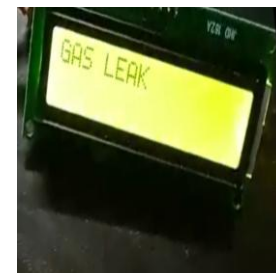
Fig. 13. Gas leakage indication on LCD
