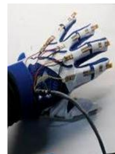
Fig. 4. Flex Sensors mounted on Gloves
