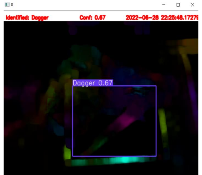
Figure 7. Detection of object followed by application of dense optical flow estimation.
