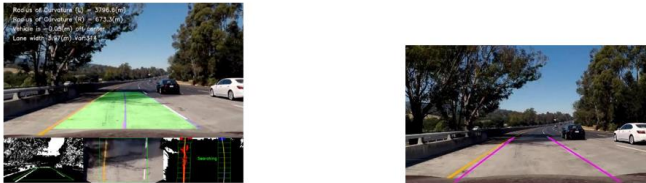
Fig 9. Our proposed algorithm on the left versus Canny and Hough transform lane detection based algorithm
