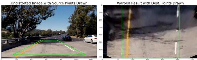
Fig 6. Shows an aerial view of the warped image lane on the right
