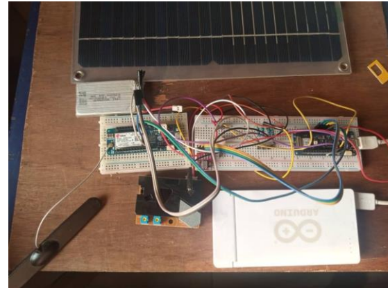
Fig. 4. Experimental set-up of the key components of the node.
