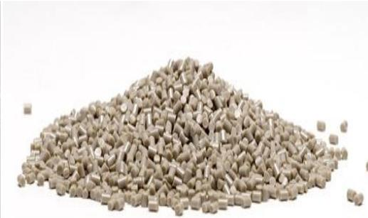
Figure 2 Pellets form of PEEK<sup>[16]</sup>
