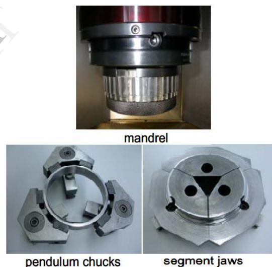
Fig. 3 Mandrel, Pendulum chuck and Segment jaws[9]
