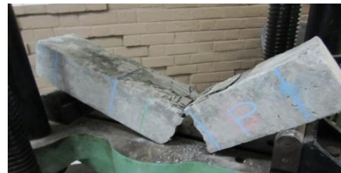
Fig.7: Cement Concrete Beam Failure
