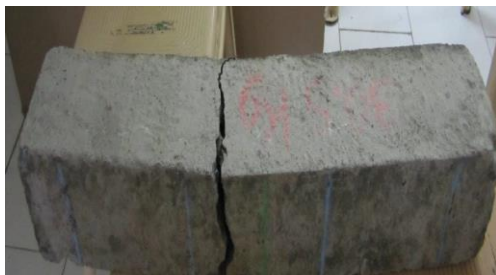
Fig.10: Failure of Singly Reinforced Beam
